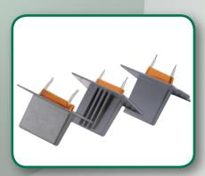
T-type PTC water heater for foot massager can heat the water in a stable temperature when immerges into a fluid container. As a heat source, this kind of PTC water heater has such advantages as warming up rapidly, constant temperature, power controlling. It enjoys a low cost and is more endurable and will not be damaged when used without water.
