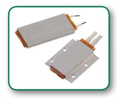
PTC heater with shell consists of one or more PTC stone(s) combined with two aluminum or stainless steel plates as electrodes and packed in insulating film and then embeds in a specially designed aluminum shell. It is designed for the self-regulated heating in a small space such as inner space of electrical equipment. No temp, thermostat is required. This type of PTC heaters is characterized as high efficiency, high reliability, safety and conveniently operation.
