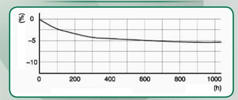
Decay rate is used for evaluating the durance of PTC heaters. According to Industry Standard, the decay rate should  $\leq$  10% after working for 1000 hours.
