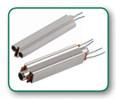
Pipe-type PTC water heater is another kind of products for foot massagers, mainly use in the high-level of foot massagers for cycle heating. Unlike another traditional heating material such as Quartz glass tube, it is easy to fit and not easy to damage which has a long service life. The power ranges from 400w to 1500w.
